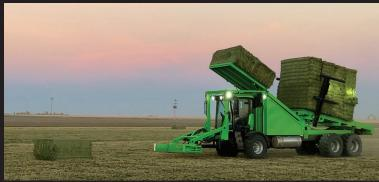
The receiving table has capabilities of lifting up to 45 degrees, this allows for stacking in tougher climate conditions. This allows the bales to slide easily without having to backup to get them to slide in heavy dew conditions.
