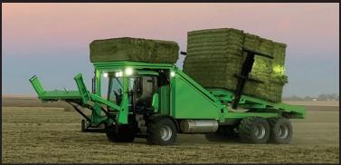
The bale alignment holds the front two bales from falling on the front table in hills and rough conditions. It aligns the bales for a consistent, even stack.
