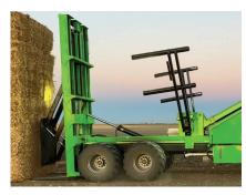
The pushoff pushes on the bottom three bales creating a tighter, straighter stack.
